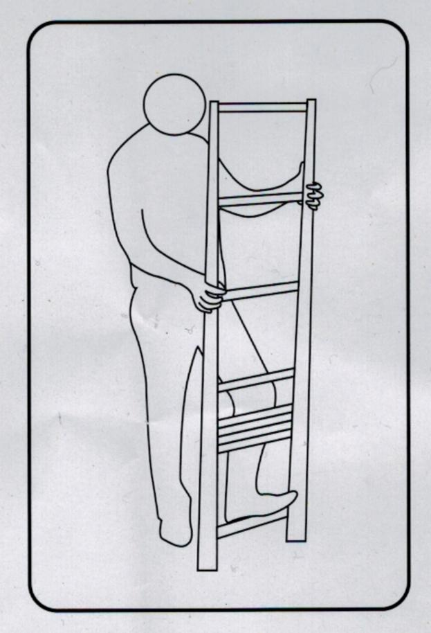
2 Grasp ladder rod by hand and the ladder will contract downwards automatically by joint one and another.
