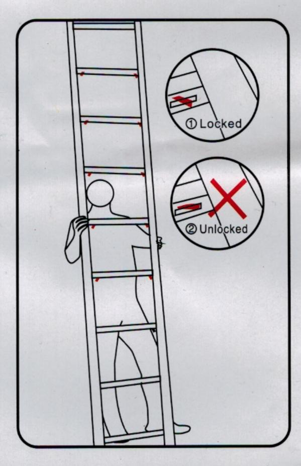
It is necessary to check wether the crosspiece is locked before using (It is locked in Figure 1 and unlocked in Figure 2), keeping from the unexpected happened. When using it, the ladder should be 75 degree between floor and ladder.
