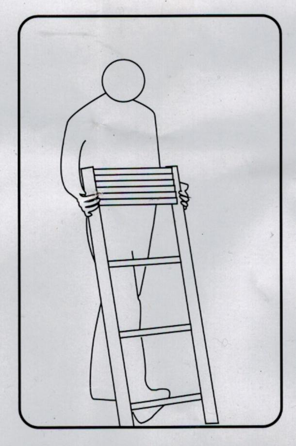
2 When open the ladder, you can step on the lowest crosspiece by one foot and lift it upwards horizontally to reach your needed height.
