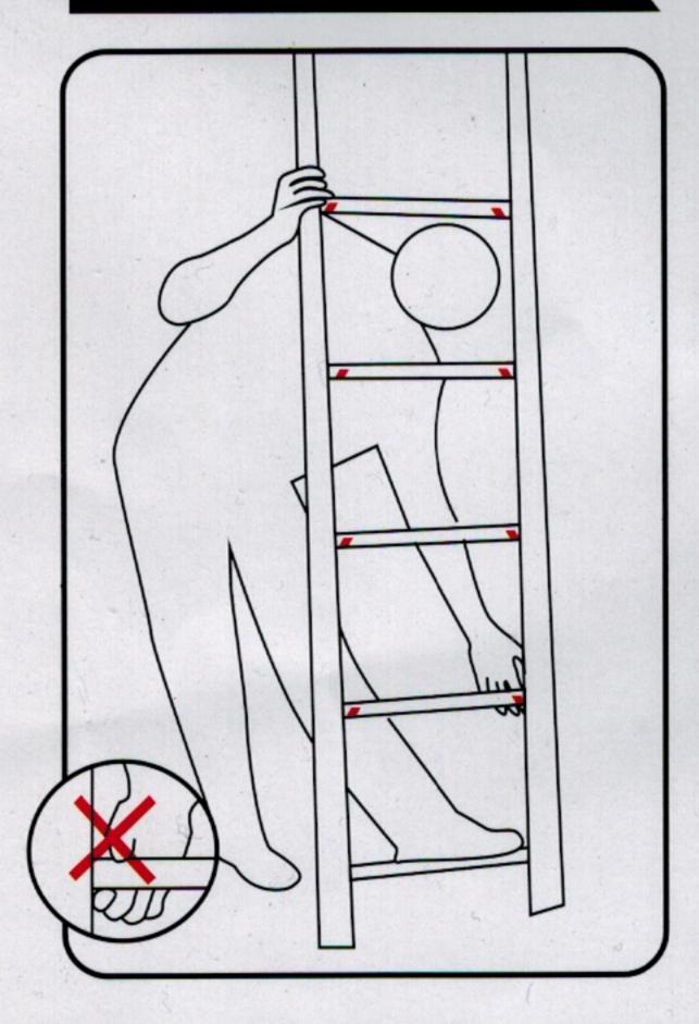
1 Step on the lowest crosspiece by one foot, grasp the ladder rod by one hand, and press the left and right switches of the lowest crosspiece. Note(Figure 3): Do not put your hands on the crosspiece when pressing the contraction switches.
